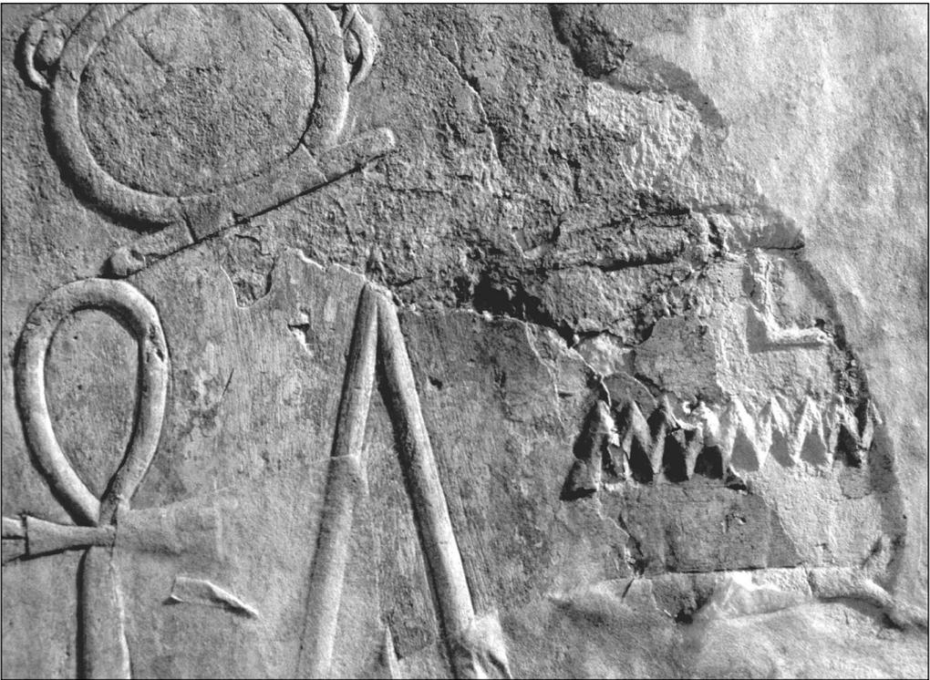
*Fig. 1. An example of exfoliation. Block without polychromy from the northern wall of the Upper Courtyard (Photo R. Gazda)*
